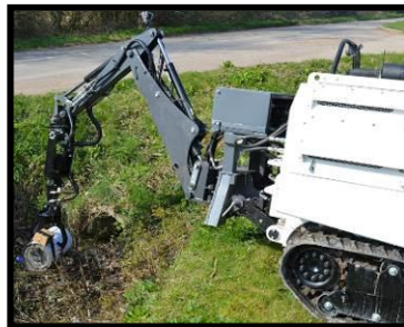
Armtrac 20T Mk2 {Small (Heavy) UGV} which is deployed in Colombia investigating a culvert IED
